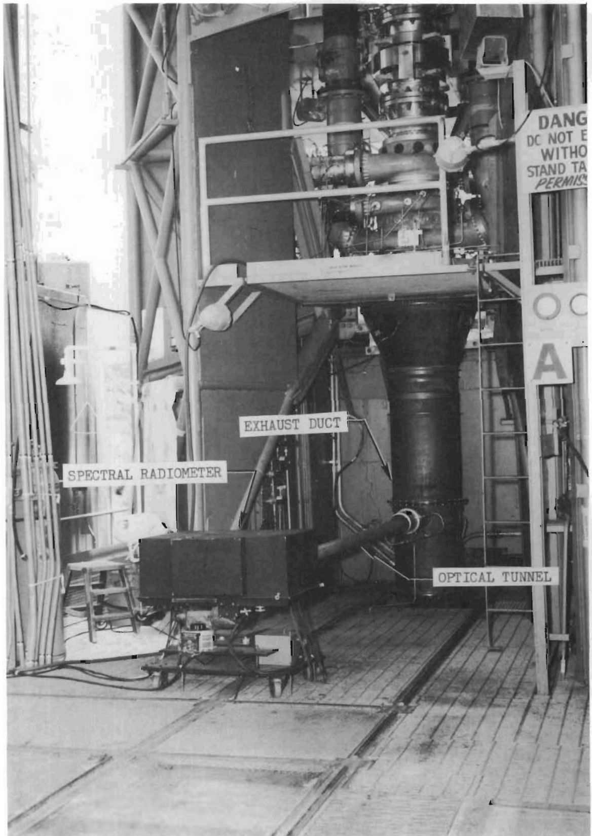
Figure 11. Spectral Radiometer Installed on Test Stand R-6743
